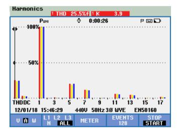
Fig: 5 Harmonics reading without SVC installed
