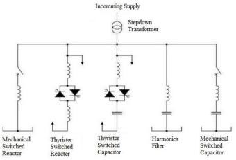
Fig: 3 Static VAR Compensator (SVC)
