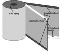
Fig: 1 construction of Metallized film capacitor (MPP)
