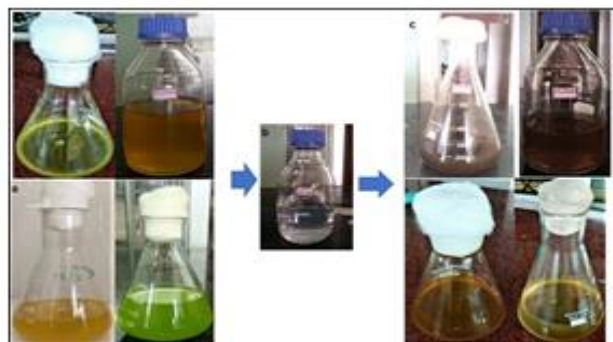
Fig. 2 Color change after the addition of algae extract with 1mm AgNO 3 indicates the formation of silver nanoparticles. (a) Microalgal extract b) silver nitrate solution c) Initial color change, (d) after 2hr
