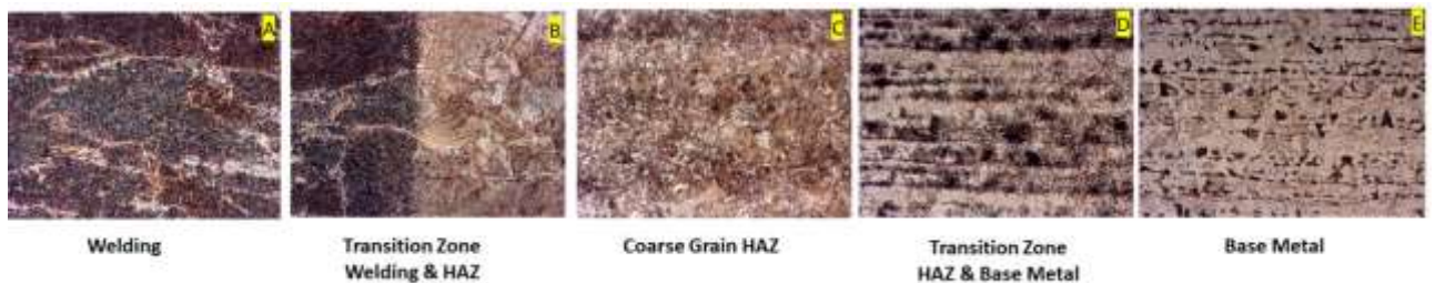
Figure 7. Microstructure study from welding to plate zone
