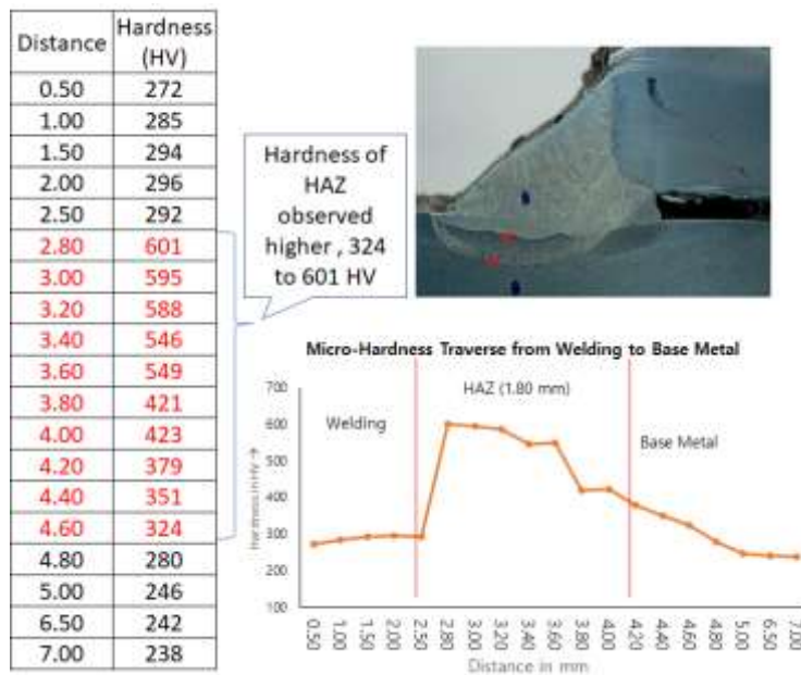
Figure 10. Without pre-heating welded sample - micro hardness observations
