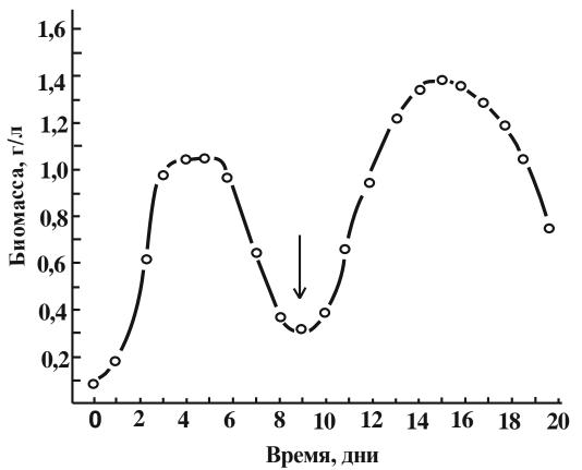
Fig. 2. Dynamics of Dunaliella salina biomass change in synchronous culture in 10 l laboratory bioreactor with illumination of 6000 - 8000 lux (108 - 144  $\mu$ Mols-1m-2) and air bubbling (5-6 l/m). The arrow shows the addition of the consumed biogenic elements concentrate (KNO3, K2HPO4) to the initial Arthari medium concentrations.
