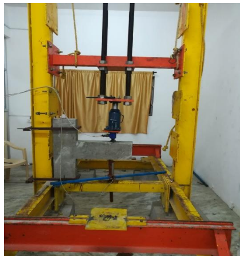
Fig 3.7- Specimen Placed On Loading Frame for Testing
