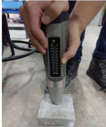
Fig 3.5 Testing of concrete by Rebound Hammer
