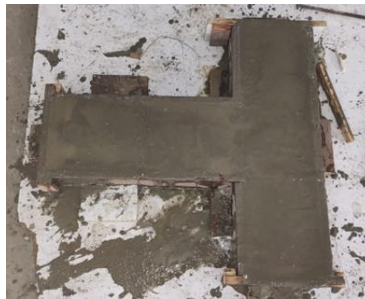
Figure3. 3 – Concreting of the specimens Testing of specimen
