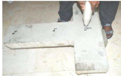
Fig 3.6- Testing of Beam column joint by Rebound Hammer
