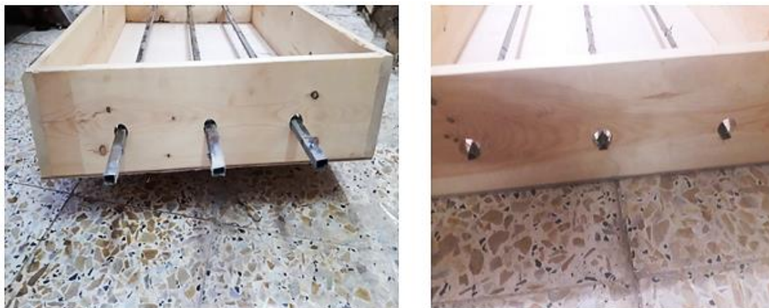
Fig. 10 Horizontal Solar Collector Containing Three Rectangle Tubes
