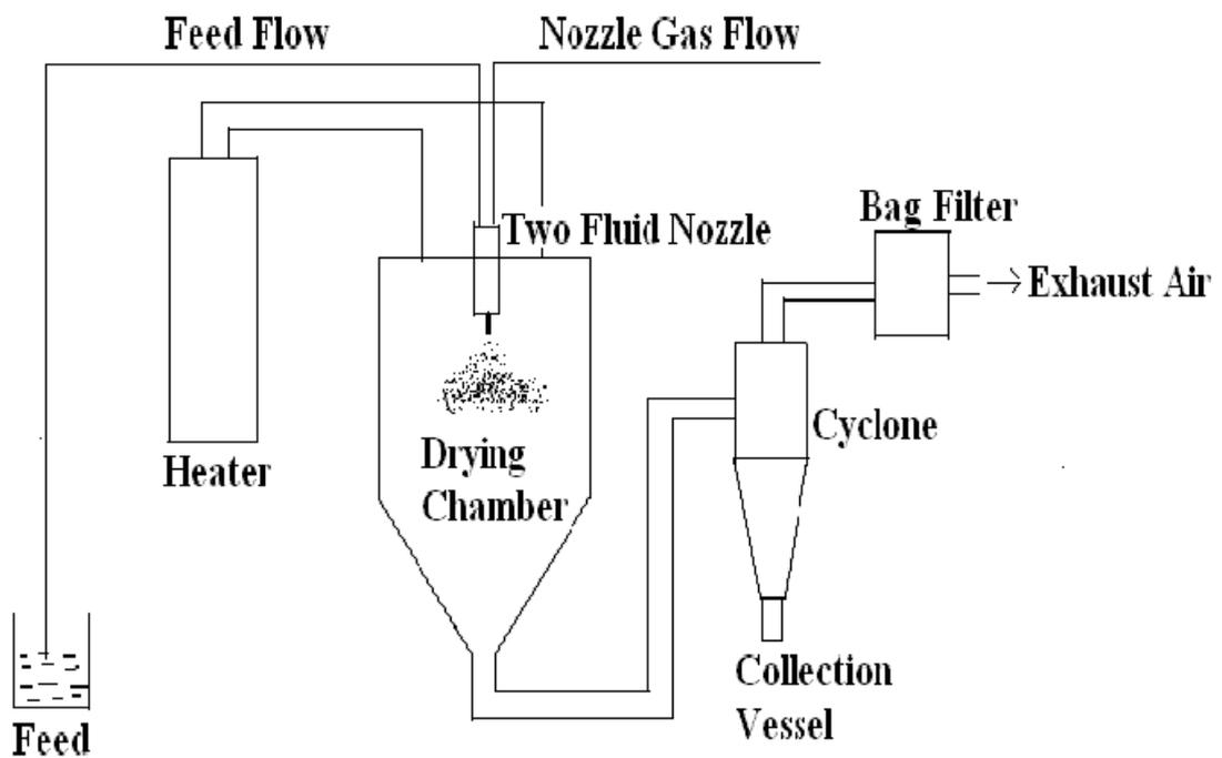
**Figure: 2 the Spray Dryer** <sup>11</sup>
