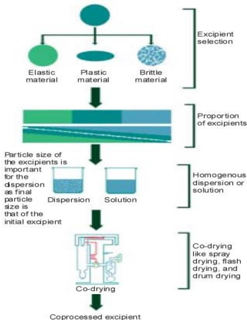
**Figure: 1** schematic representation of steps involve in co-processing<sup>6</sup>
