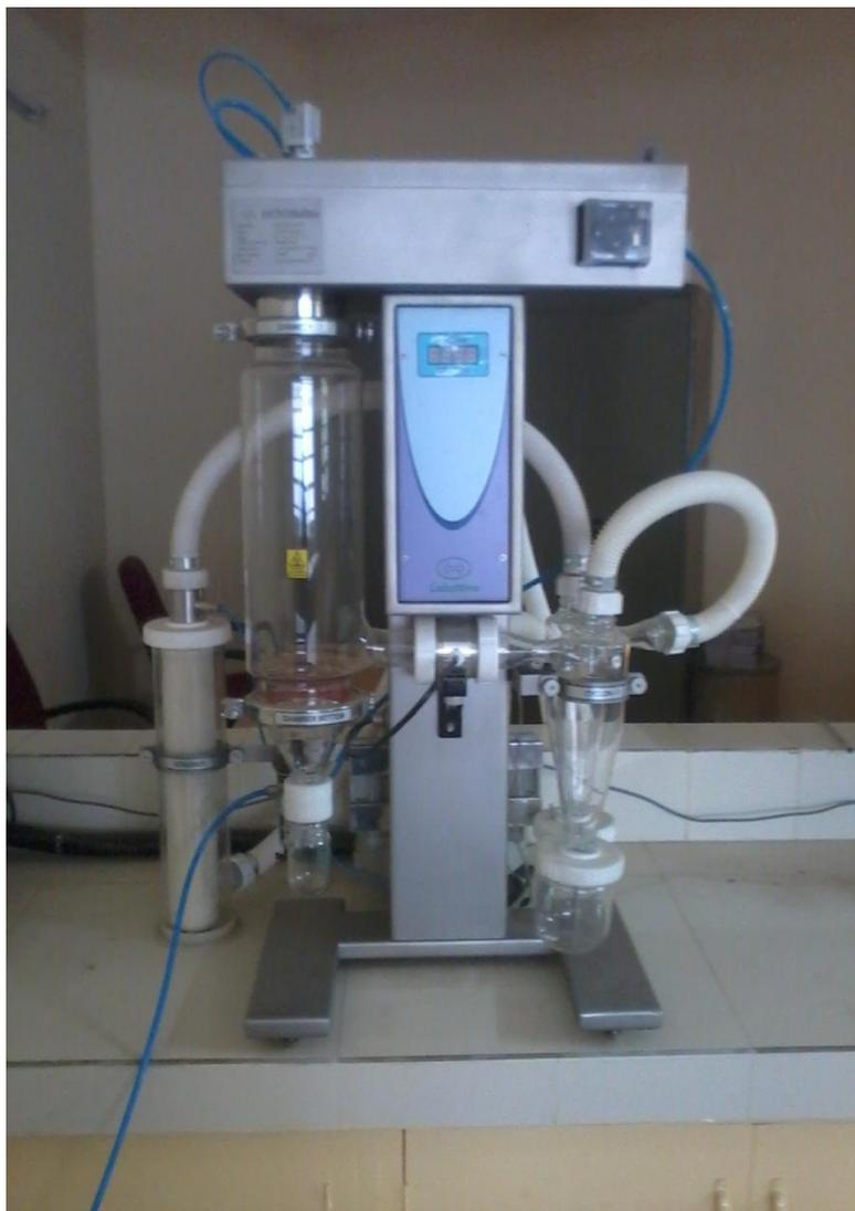
**Figure: 2 the Spray Dryer Lab spray dryer (EU 222 advanced) Electrolabultima**
