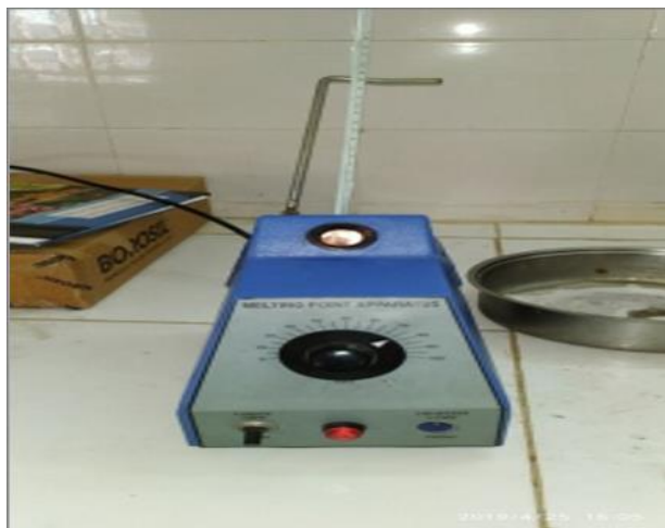
Fig 1. Melting point test through melting point apparatus.
