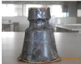
Fig.25. Epoxy coated insulator
