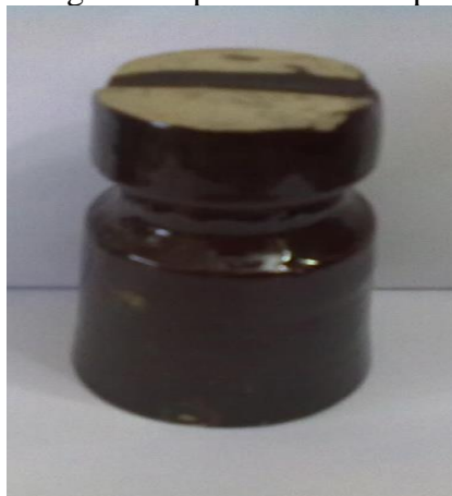
Fig.18. Pin type insulator model
