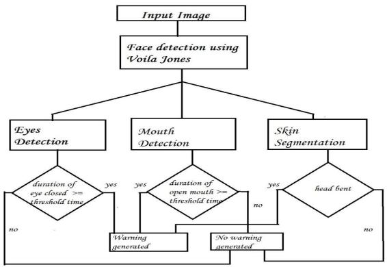
Fig 1: Flow Diagram for working of the detection system
