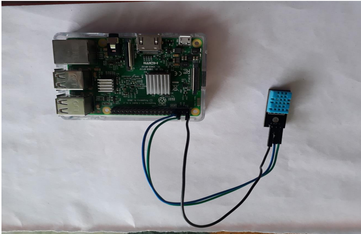
Figure 6 implementation of the temperature and humidity sensor with raspberry pi
