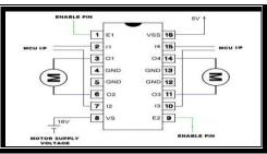
Fig 1.3 L293 Driver circuit
