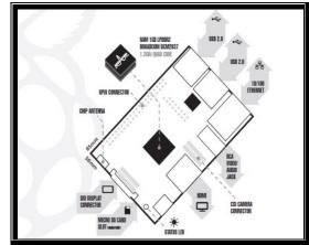
Fig 1 Architecture of Raspberry pi
