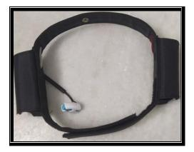
Fig 1.2 Brain wave detecting headset
