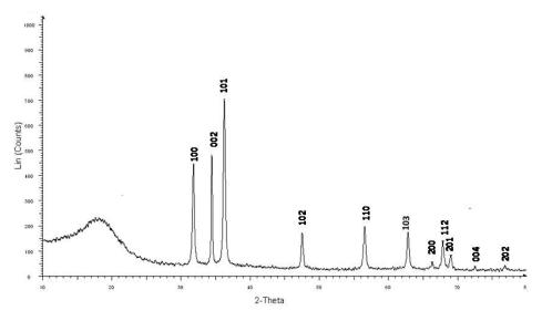
Fig.1 XRD pattern of ZnO NPs mediated by WRE
