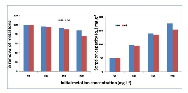
Fig.3 Plots of percentage removal and loading capacity of synthesized ZnO NPs towards Pb2+ and Cd2+ ions from aqueous solution
