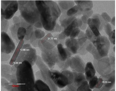
Fig.2 TEM image of synthesized ZnO NPs mediated by WRE
