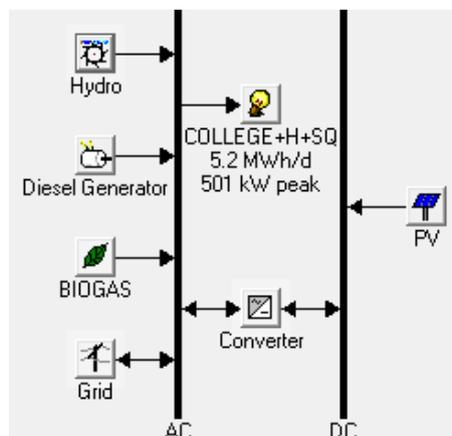
Figure 3. Grid/diesel generator/PV/Biogas/SHP
