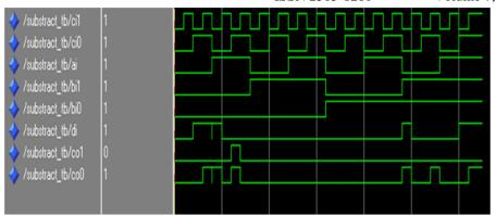
Figure.5. Subtract Simulation results
