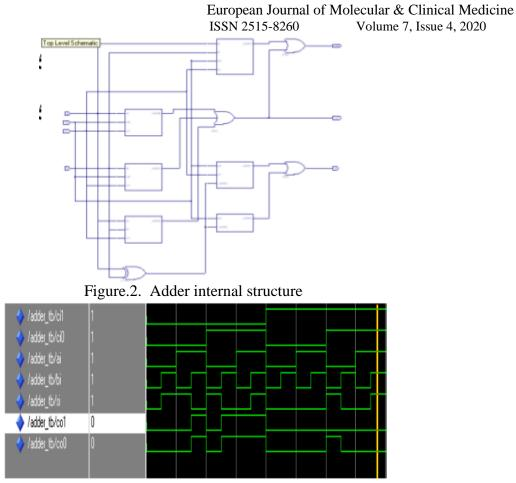
Figure.3. Adder Simulation results
