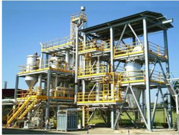
The 500 KW e FICFB gasifier at Trisaia.
