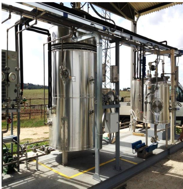
Fig. 7 Two-stage anaerobic digestion pilot plant at CREA Research Centre [15]
