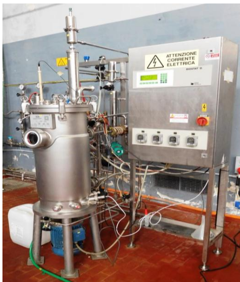
Fig. 8 Pilot fermenter (50 L) at ENEA Trisaia Research Centre [16]
