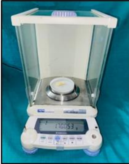
Fig. 4- weighing of control model using microbalance
