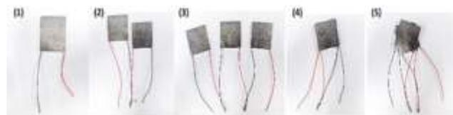
Figure 3: Different TEG connections: (1) single TEG, (2) two TEG series, (3) three TEG series, (4) two TEG parallel and (5) three TEG parallel
