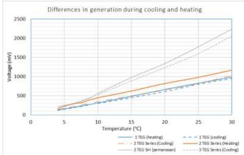
Figure 11: Performance Comparison between Heating and Cooling
