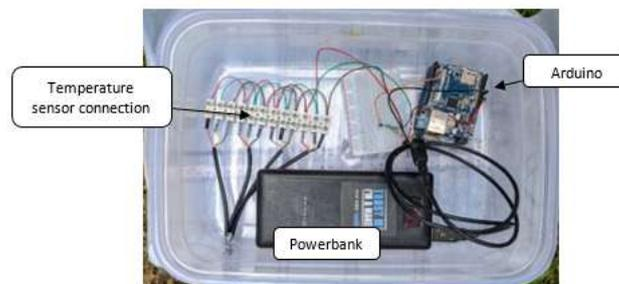
Figure 1: Temperature collector model
