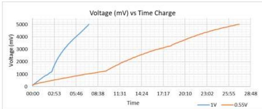
Figure 13: Time taken to fully charge Super capacitor
