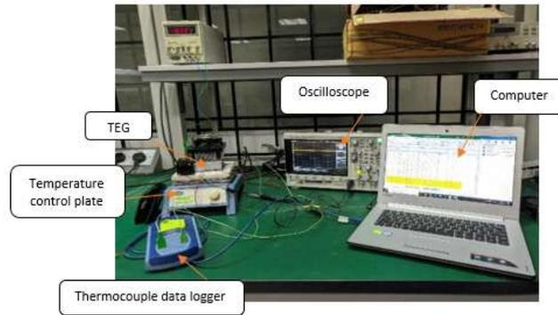
Figure 4: Actual test setup for TEG testing
