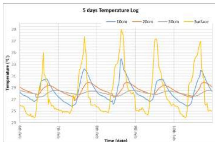
Figure 7: Temperature of Soil in various depth
