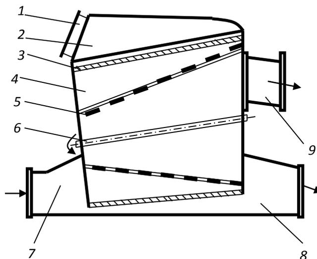
Figure 4. Separator with a conical mesh shell drum
