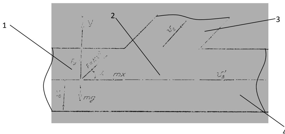
Figure 6. The movement of cotton in the separation zone of the horizontal pipe (1) horizontal pipe to the separation zone; Separation zone (2); (3) oblique tubes; (4) horizontal pipe after separation zone.
