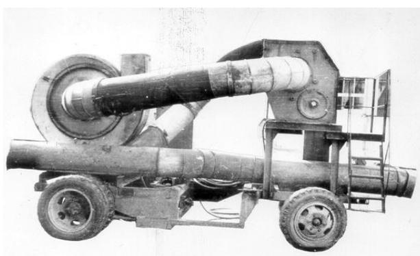
Figure 5. A moving device with a separation zone in a horizontal pipe
