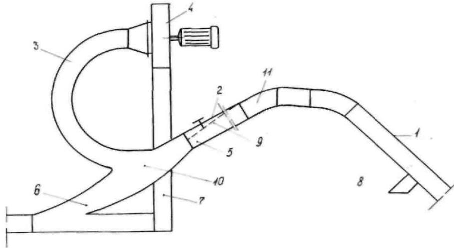
Figure 2. Pneumo separator
