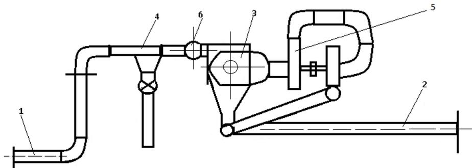
Figure 1. Pneumatic transport device of ‘Hard Wick – Etter’ (1) and (2) suction and drive pipes, (3) separator, (4) stone holder, (5) fan, (6) electromagnet.
