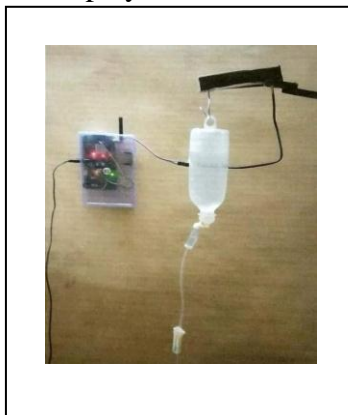
Fig 1.3 b) Hardware implementation of the proposed system installed in infusion bottles. In Fig 1.3 b) our prototype is installed in the drip infusion bottles which is used in the hospitals for patients who are bed ridden.
