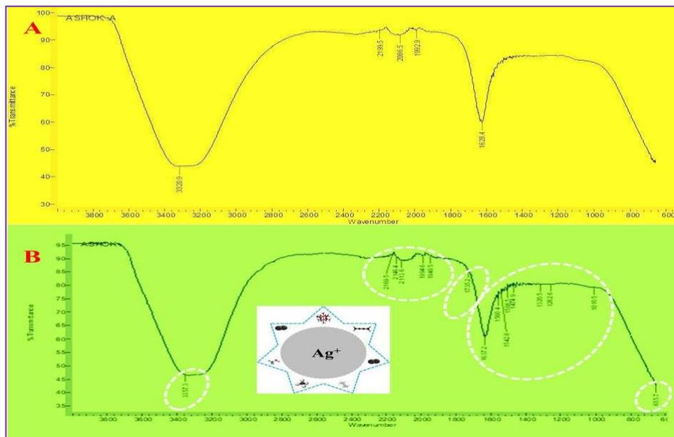
**Figure 2:** FTIR spectrum of A- *A. hypogaea* RN AE and B- Green synthesized AgNPs (dotted white circle highlights the functional groups responsible for the bioreduction)
