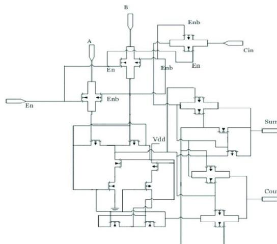
Fig. 2 Existing self-latching Full-Adder Schematic
