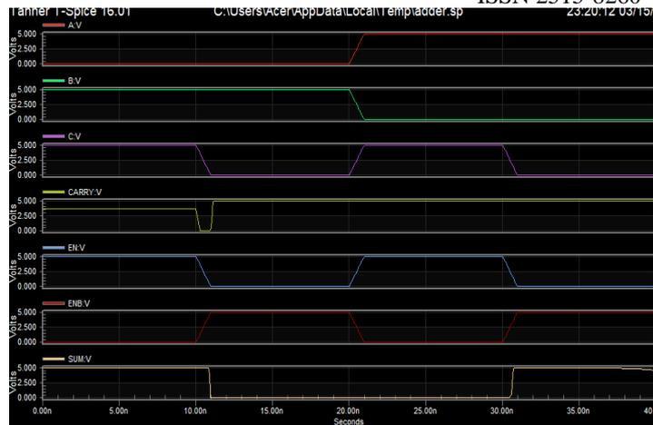
Fig 14 : full adder waveforms schematic
