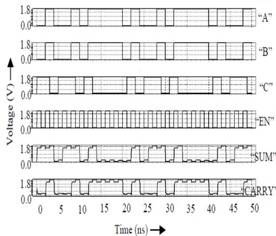
Fig.3 Transient I/O response of self-latching Full-Adder
