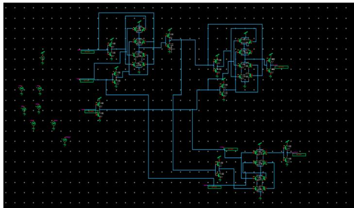
Fig 15 : XOR based multiplier schematic
