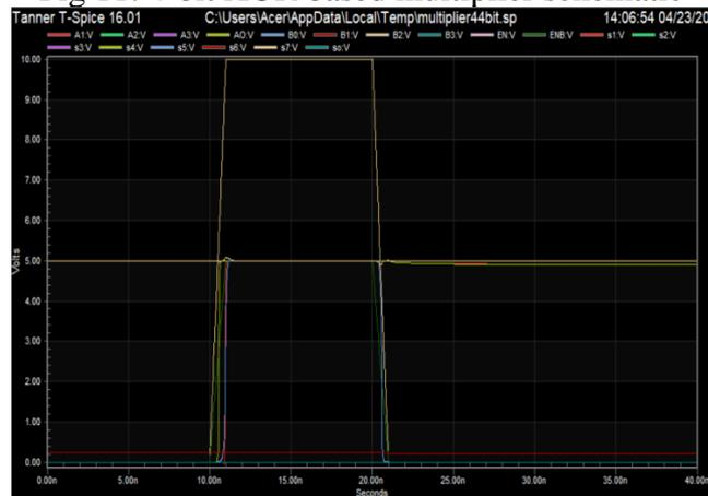
Fig 12 : 4-bit XOR based multiplier waveform
