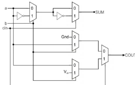
Fig 6 : Full adder realization predominantly based on 2:1 MUX
