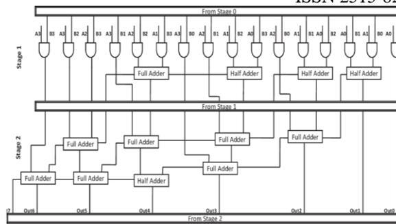
Fig.4 Existing 4-b×4-b Self-pipelined multiplier Schematic
