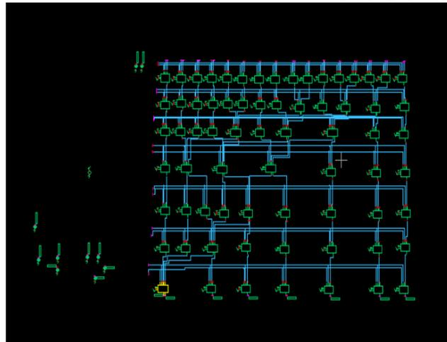
Fig 11: 4-bit XOR based multiplier schematic
