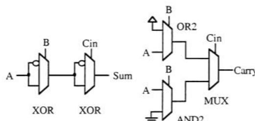
Fig. 5. Sum and carry based on 2-1 MUX circuits
