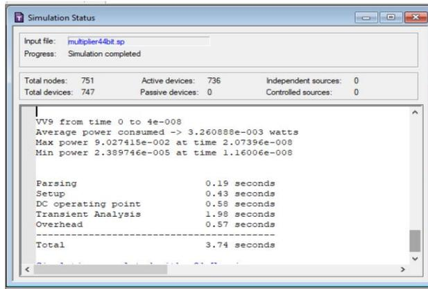
Fig 8: 4 bit XOR based multiplier simulation
