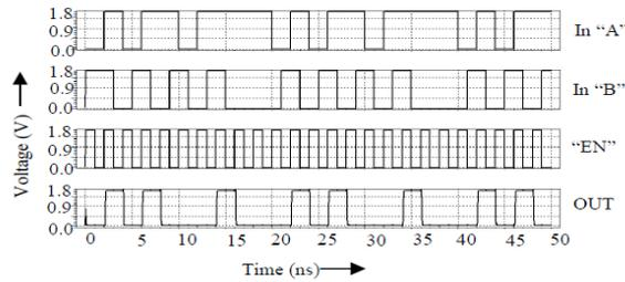
Fig. 1 Transient response of Latch-AND
