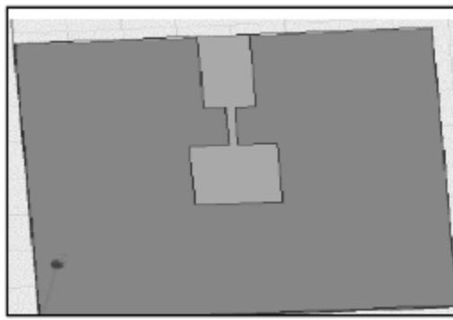
Fig 8: Square type-2 Antenna with stub feedline
