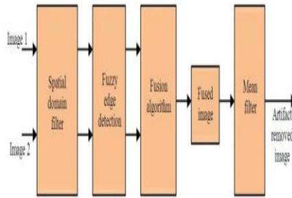
**Fig. 1. Block diagram of proposed fusion methodology**
