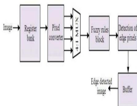
**Fig. 3. Architecture of fuzzy based edge detector**
