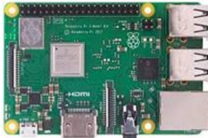
*Figure 2:Raspberry Pi 3 Model B+*
