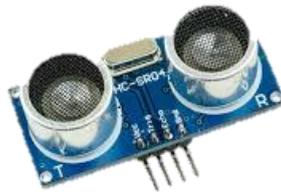
*Figure 5: HC-SR04 ULTRASONIC SENSOR*
