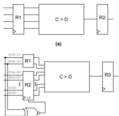
Figure 1. Precipitation Applied to a Comparator
