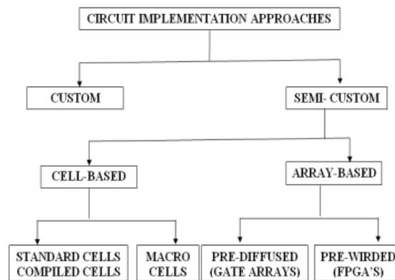
Fig.2: Overview of Implementation approaches for Integrated Circuits
