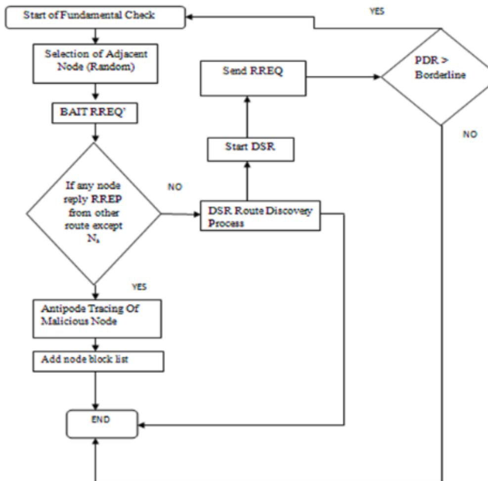
Figure 3.2 Operation process of CBD technique
