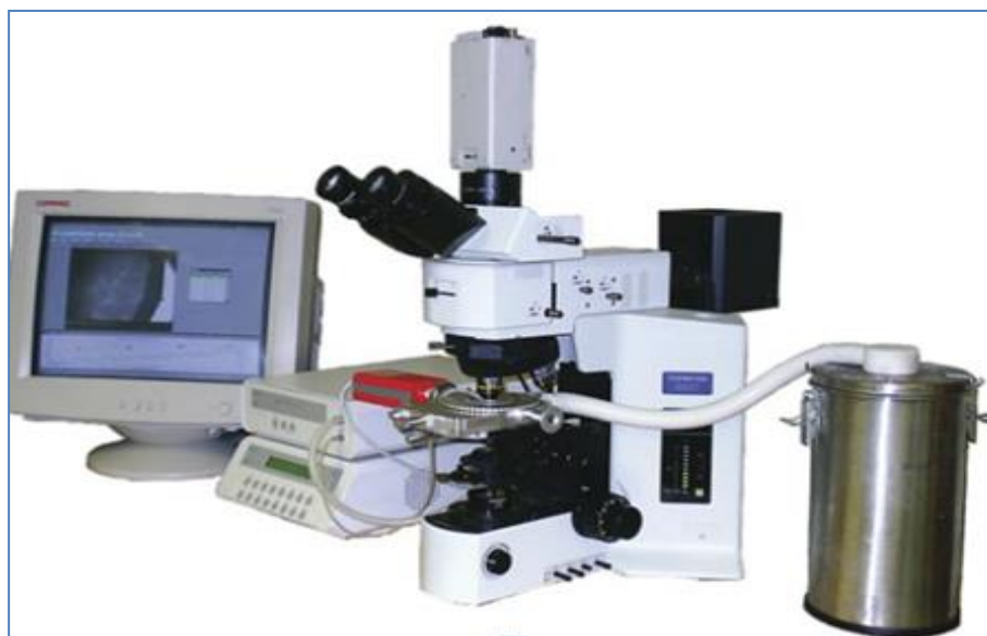
Figure 2: Typical Set up of Freeze Drying Microscope
