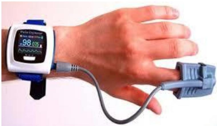
**Figure 3: Fingertip pulse analysis wearable device**
