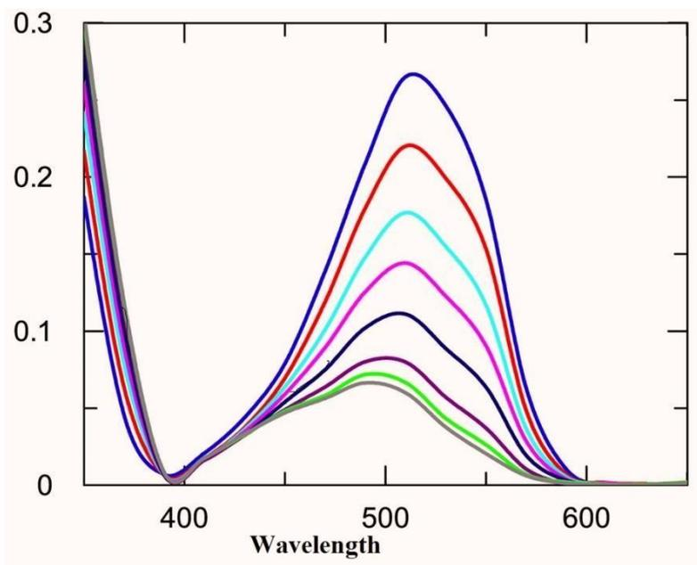
**Fig. 7. UV visible spectra Degradation of Methyl red dye using Plant assisted aluminum oxide nanoparticles.**
