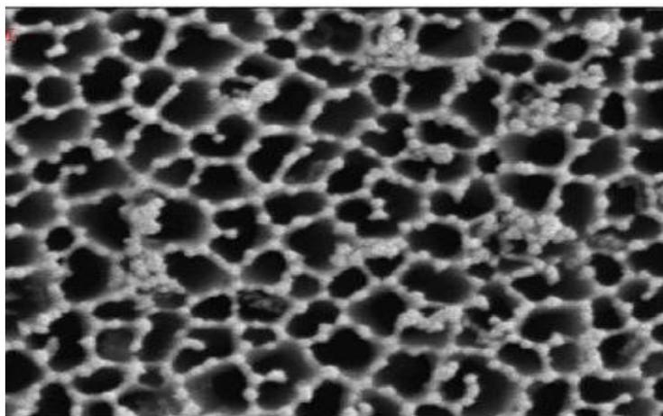
**Fig. 3. Image of SEM of Plant assisted aluminum oxide nanoparticles**
