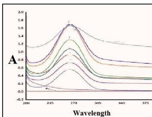
**Fig. 6. UV visible spectra Degradation of Congo red dye using Plant assisted aluminum oxide nanoparticles.**
