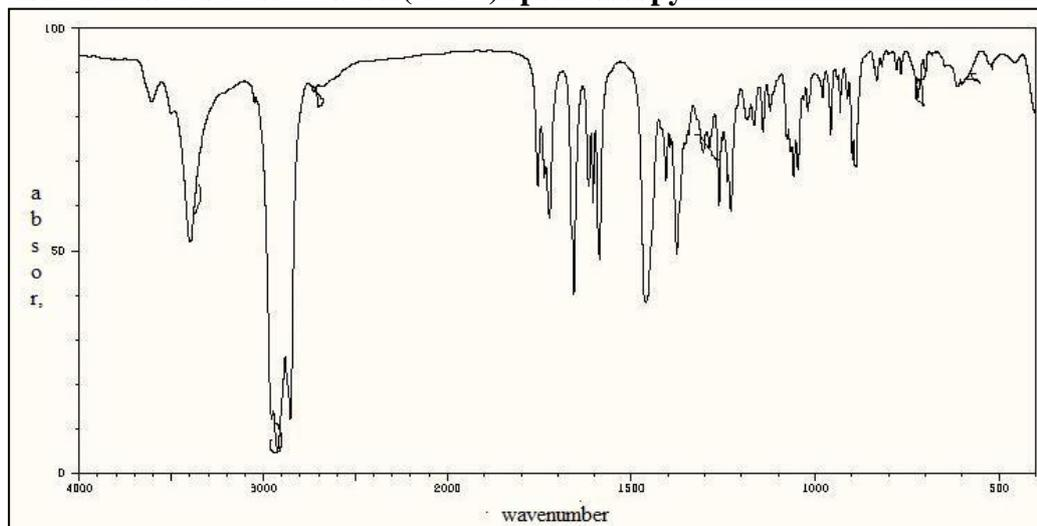
**Fig. 2. Fourier transforms infrared (FTIR) spectra of Plant assisted aluminum oxide nanoparticles.**
