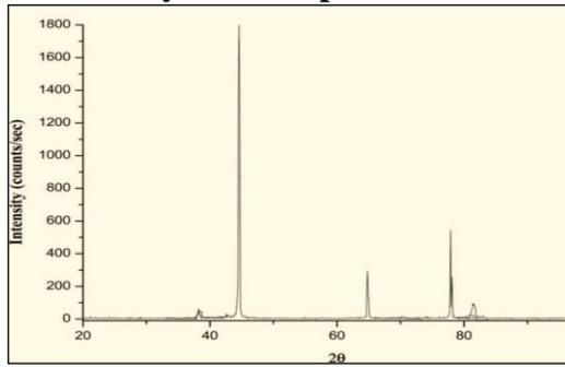
**Fig. 5. XRD Analysis of Plant assisted aluminum oxide nanoparticles.**
