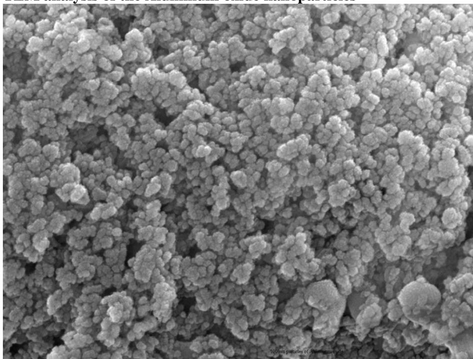
**Fig. 4. TEM analysis of Plant assisted aluminum oxide nanoparticles.**
