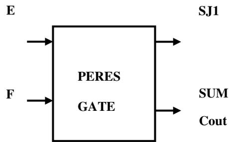
Fig. 13. Peres Gates as Reversible Half Adder
