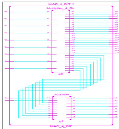
Figure 5: RTL Schematic of 4-Bit MAC
