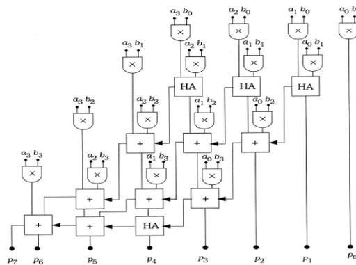
Figure 2: 4 Bit Array Multiplier
