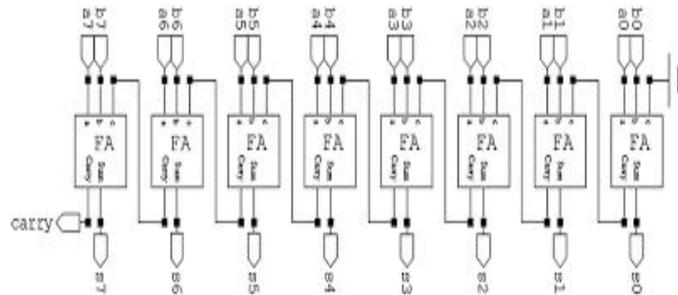
Figure 3: 8-Bit Ripple Carry adder
