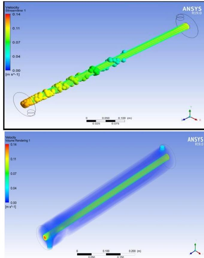
Fig-6 velocity flow in Tube in Tube, Acetoacetate /Water as a Fluid
