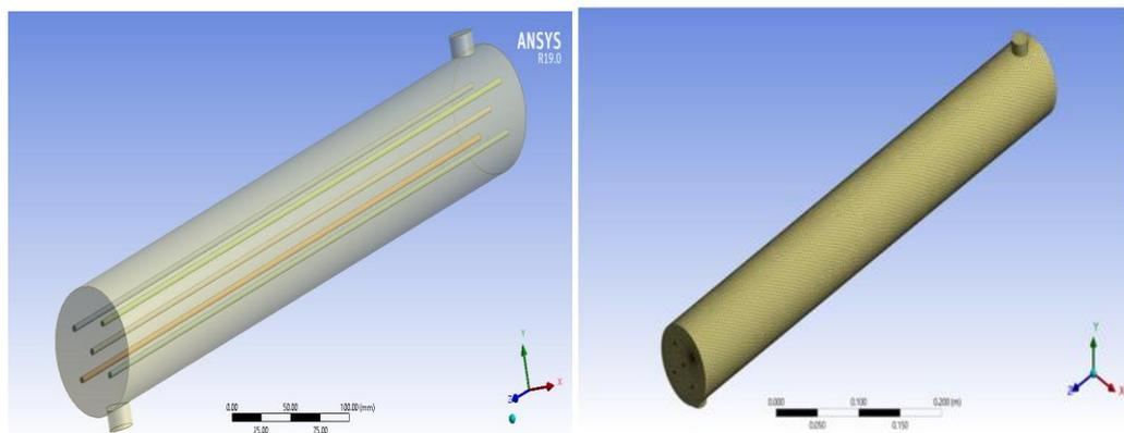
Fig-1 geometry and meshing of shell and tube heat exchanger
