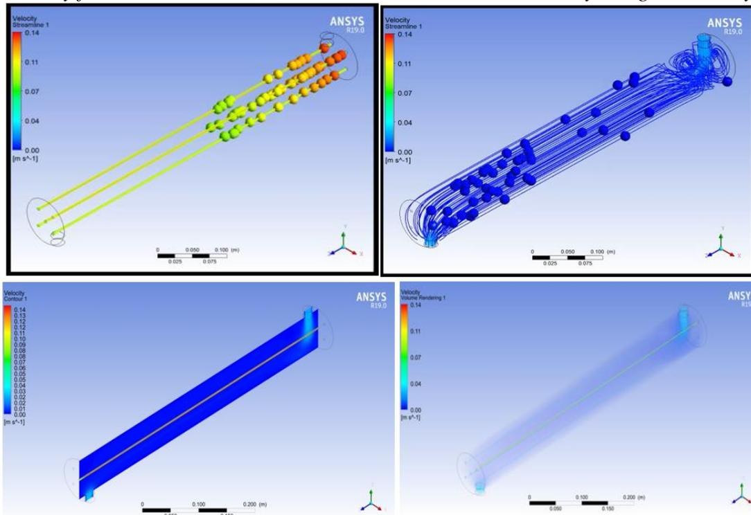
Fig-5 velocity flow in Shell and Tube, Acetoacetate /Water as a Fluid.
