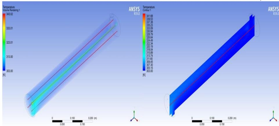
**Fig-3** Distribution of Temperature in Shell and Tube, Acetoacetate /Water as a Fluid.
