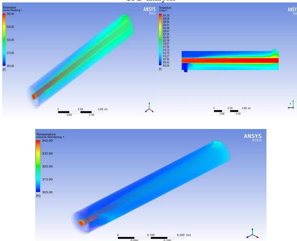
**Fig-4** Distribution of Temperature in Tube in Tube, Acetoacetate /Water as a Fluid.
