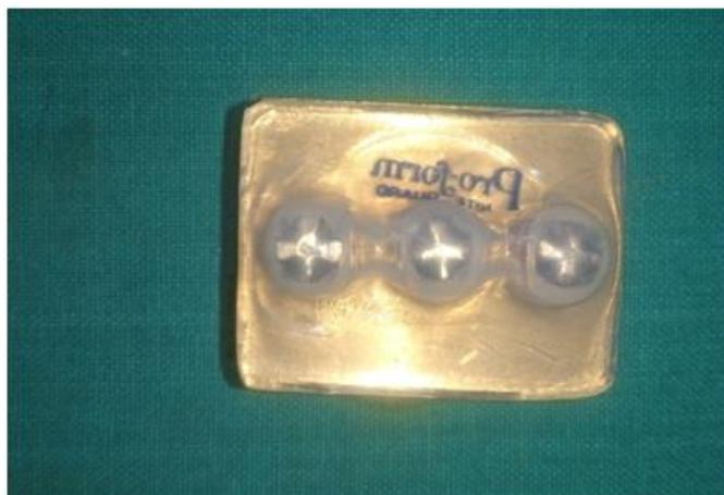
Figure 7: Stainless Steel Precision die with spacer (2 mm)
