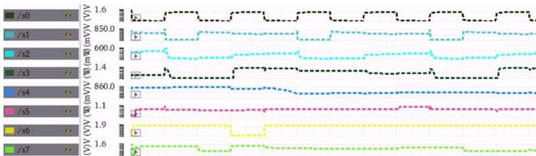
Fig. 17 Output waveform of 4 bit multiplier
