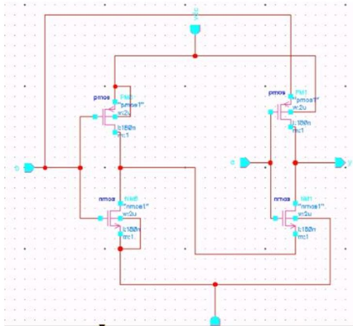
Fig. 12 Schematic output of GDI- XOR gate
