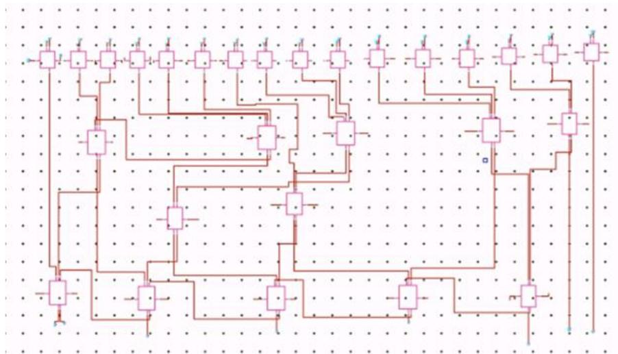
Fig. 6 4\*4 Vedic multiplier schematic
