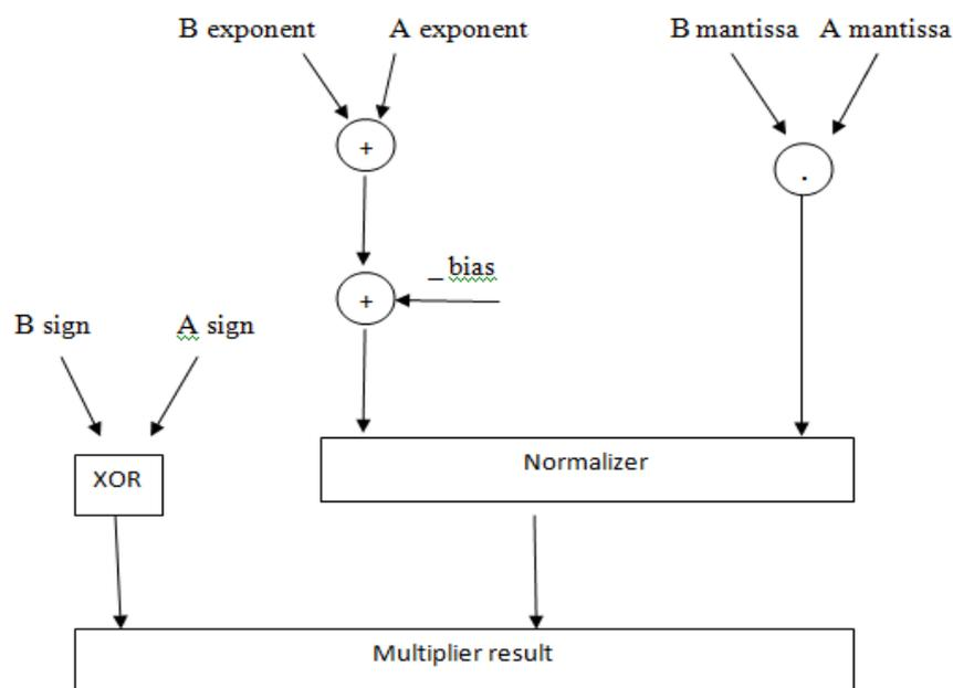
Fig. 3 Floating point multiplier block diagram
