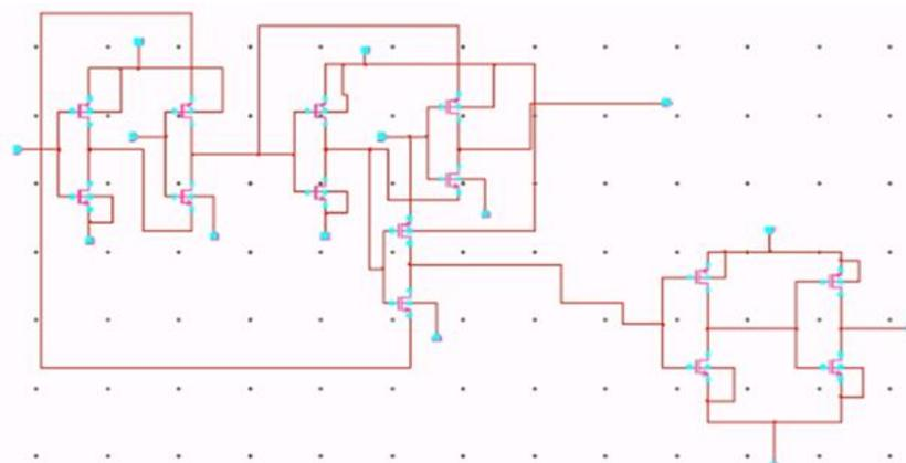
Fig. 14 Schematic output of GDI based full adder
