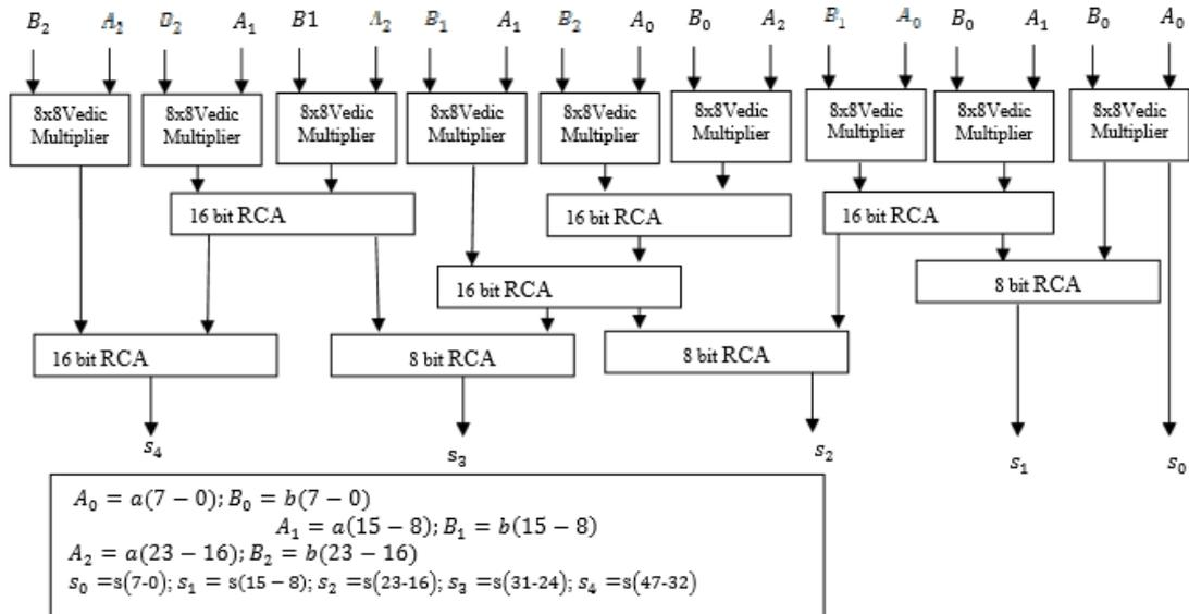
Fig: 9 24 bit multiplier architecture
