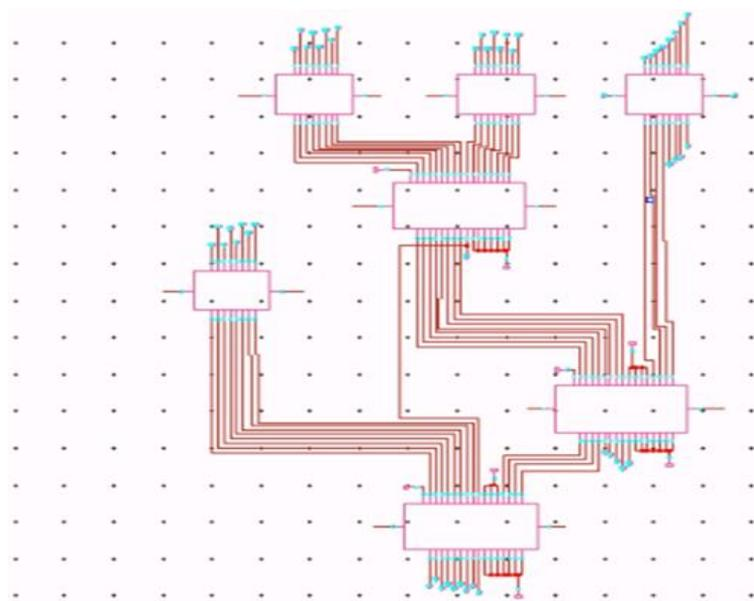
Fig. 8 Schematic of 8\*8 multiplier
