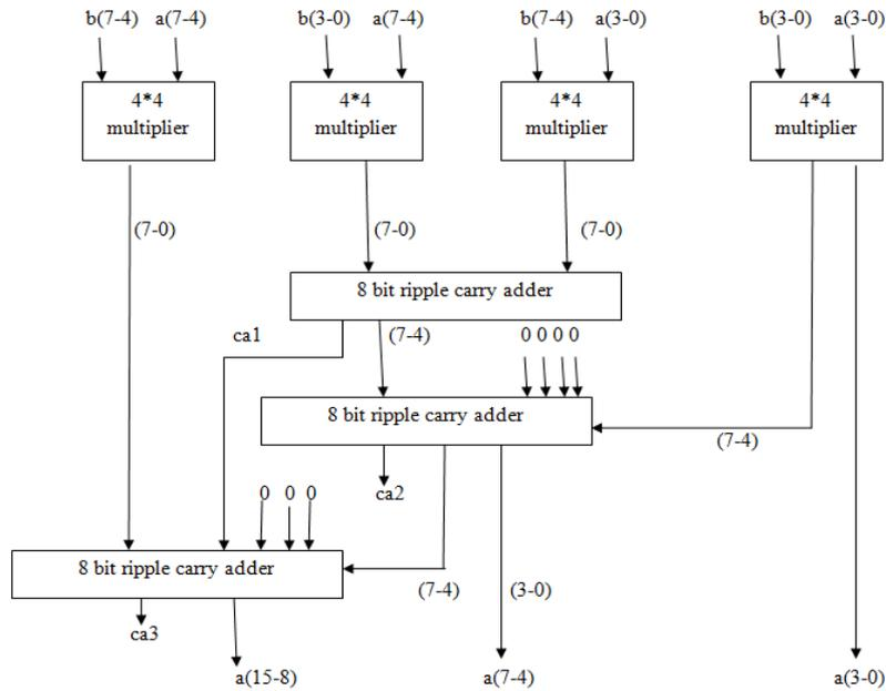
Fig. 7 design of 8 bit Vedic multiplier
