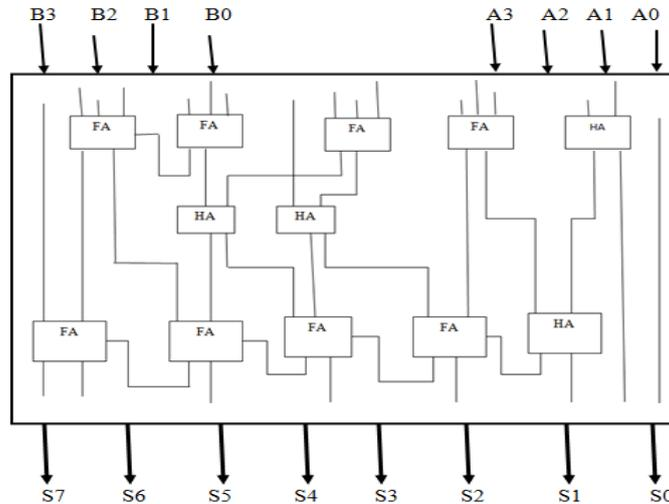
Fig. 5 Architecture of 4 bit Vedic multiplier
