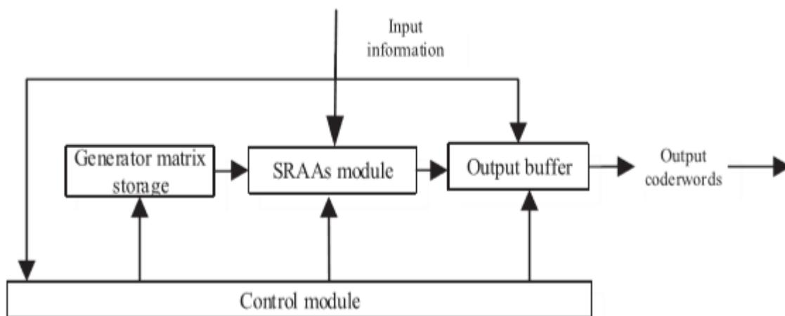
Figure 1: construction of the LDPC coding based byChinese Digital Radio.
