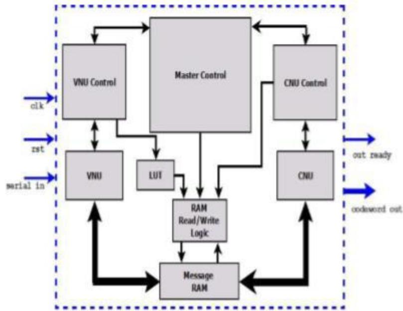
Figure 3: LDPC decoder architecture.
