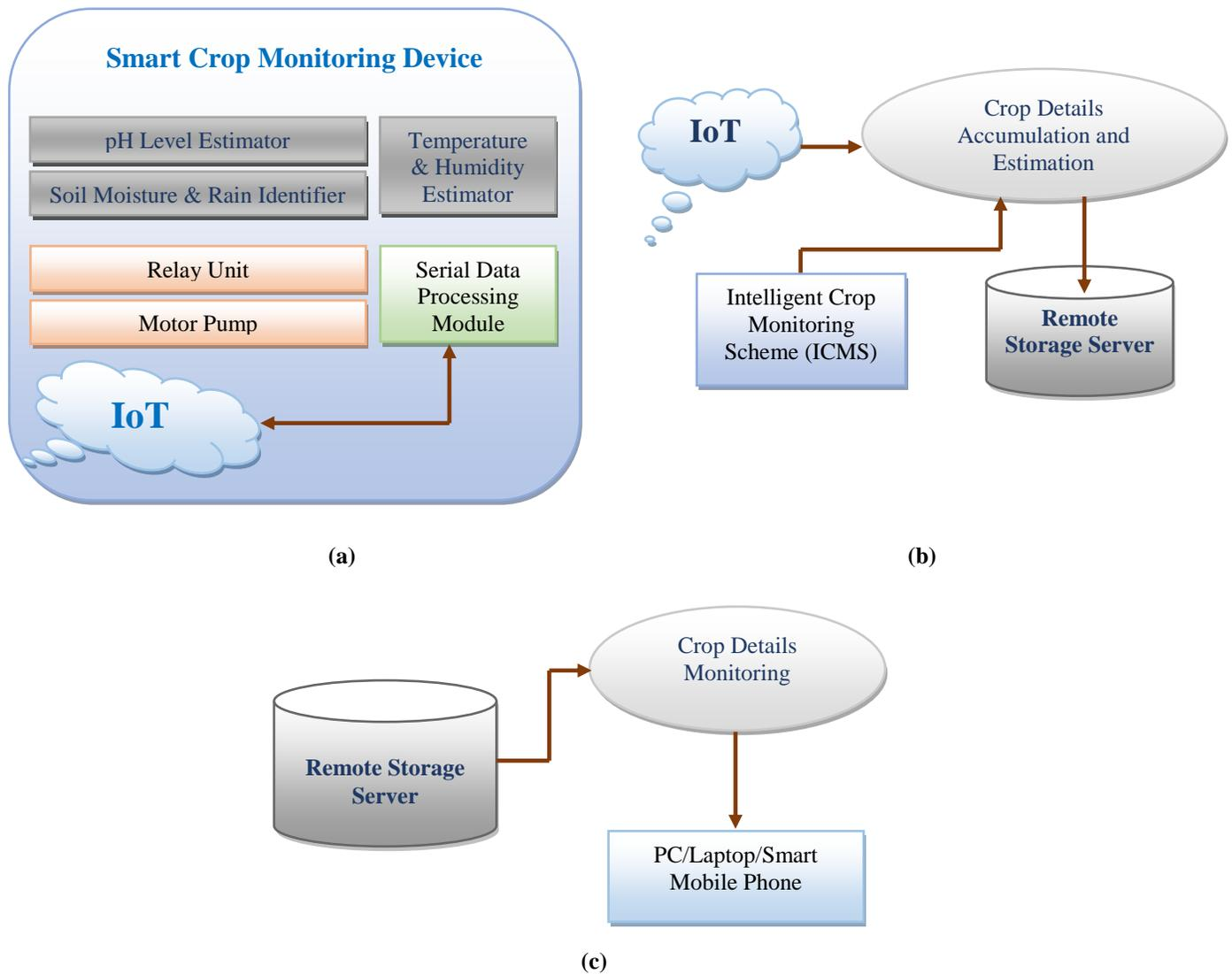
**Fig.2 Proposed Approach Architectural Design (a) Transmission and Master Smart Device block, (b) Server Processing Module w.r.t. ICMS and (c) Receiver end Monitoring and Controlling System.**
