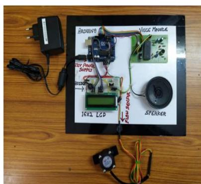
Figure 2: Output of hardware circuit
