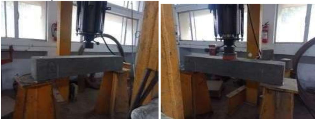
**Figure 5 Experiment test set up and point loading arrangement**
