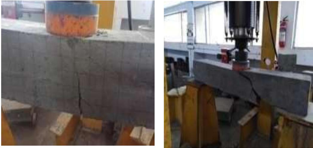
**Figure 6 Control beam with crack and failure pattern**
