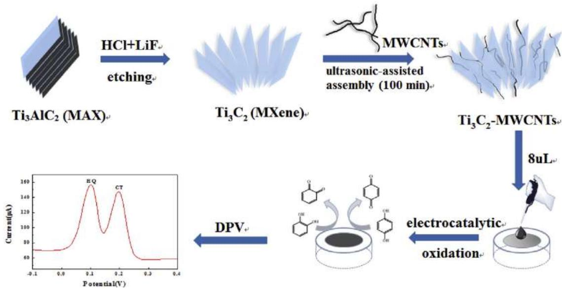
Fig.7. Schematic representation of synthesis process of  $Ti_3C_2$ -MWCNTs nanocomposite for detecting HQ and CT. Reprinted by permission from Ref. [65] Copyright 2019, Elsevier.
