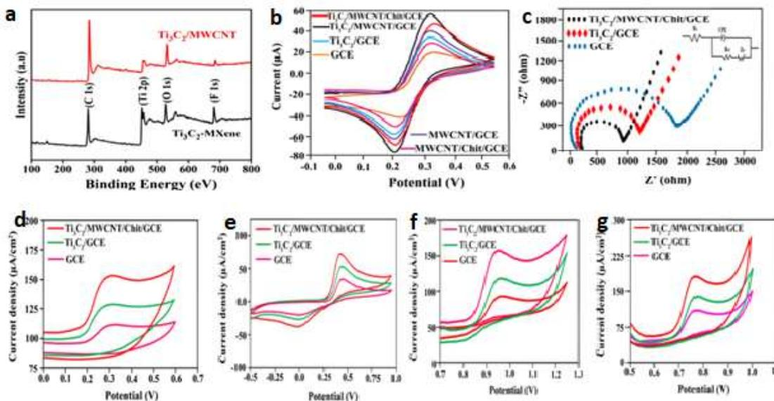
Fig.5 (a) XPS spectra of Ti<sub>3</sub>C<sub>2</sub> and Ti<sub>3</sub>C<sub>2</sub>/MWCNT (b) Cyclic voltammograms and (c) Nyquist plots of GCE, Ti<sub>3</sub>C<sub>2</sub>/GCE, Ti<sub>3</sub>C<sub>2</sub>/MWCNT/GCE, and Ti<sub>3</sub>C<sub>2</sub>/MWCNT/Chit/GCE. Cyclic voltammogram of IFO (d), ACOP (e), DOM (f), SUM (g) on the surface of these electrodes. Reprinted by the permission from Ref. [54], Copyright 2020, Springer Nature.
