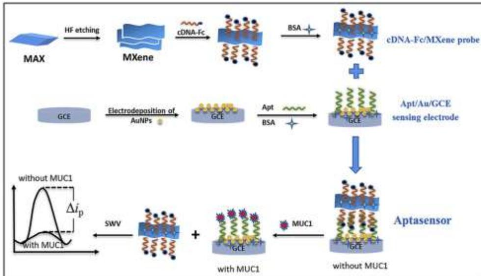
**Fig.2.** Schematic representation of the manufacture procedure of electrochemical aptasensor for identification of cancer marker MUC1. Reprinted by permission from Ref. [48]. Copyright 2020, Elsevier.
