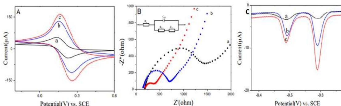
Fig.6. (A) Cyclic Voltammograms of plain GCE (a),  $Ti_3C_2Tx/GCE$  (b) and  $BiNPs@Ti_3C_2Tx/GCE(c)$ ; (B) EIS spectra of plain GCE (a),  $Ti_3C_2Tx/GCE$  (b) and  $BiNPs@Ti_3C_2Tx/GCE$  (c); (C) SWASV curves of  $Pb^{2+}$  and  $Cd^{2+}$  at GCE (a),  $Ti_3C_2Tx/GCE$  (b) and  $BiNPs@Ti_3C_2Tx/GCE$  (c). Reprinted by permission form Ref. [55]. Copyright 2020, Nanomaterials.
