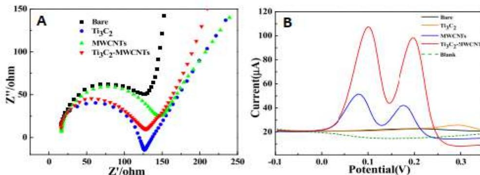
Fig.8. (A) Nyquist plots of  $Ti_3C_2$ /GCE, MWCNTs/GCE, bare GCE and  $Ti_3C_2$ -MWCNTs/GCE) (B) DPV response of  $Ti_3C_2$ /GCE, MWCNTs/GCE, bare GCE and  $Ti_3C_2$ -MWCNTs/GCE within the presence and absence of HQ and CT. Reprinted with permission from Ref. [65] Copyright 2019, Elsevier.
