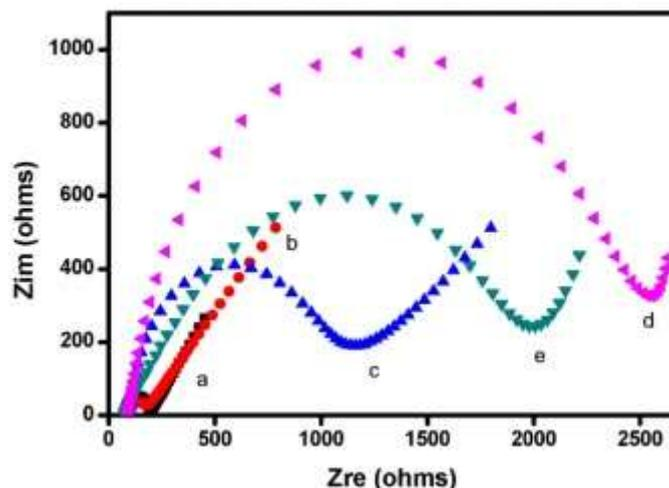
**Fig.3.** EIS spectra of different electrodes (a) GCE, (b) Au/GCE, (c) Apt/Au/GCE, (d) cDNAFc/MXene/Apt/Au/GCE and (e) MUC1/Apt/Au/GCE. Reprinted by permission from Ref. [48]. Copyright 2020, Elsevier.
