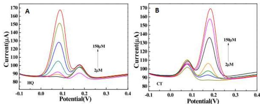
Fig.9. DPV responses of HQ(A) and CT(B) at various concentrations (2, 5, 10, 20, 50, 100, 150  $\mu$ M) in the presence of 20  $\mu$ M CT and 20  $\mu$ M HQ respectively. Reprinted by permission from Ref. [65] Copyright 2019, Elsevier.
