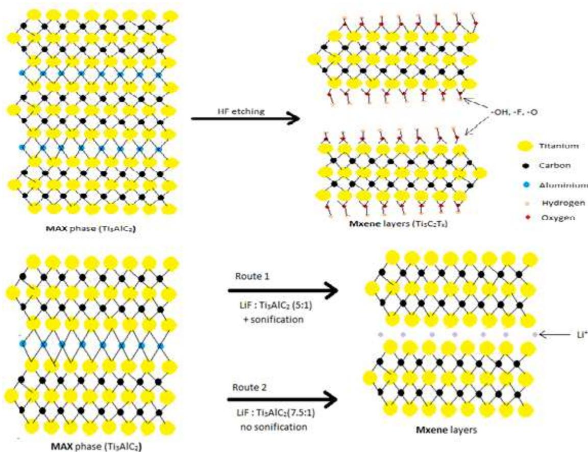
**Fig.1.** (a) Synthesis of MXene from MAX phase by using HF etchant. (b) Synthesis of MXene nanosheets through non-HF etching (generally hydrochloric acid and metal fluoride mixture is used) with and without sonification
