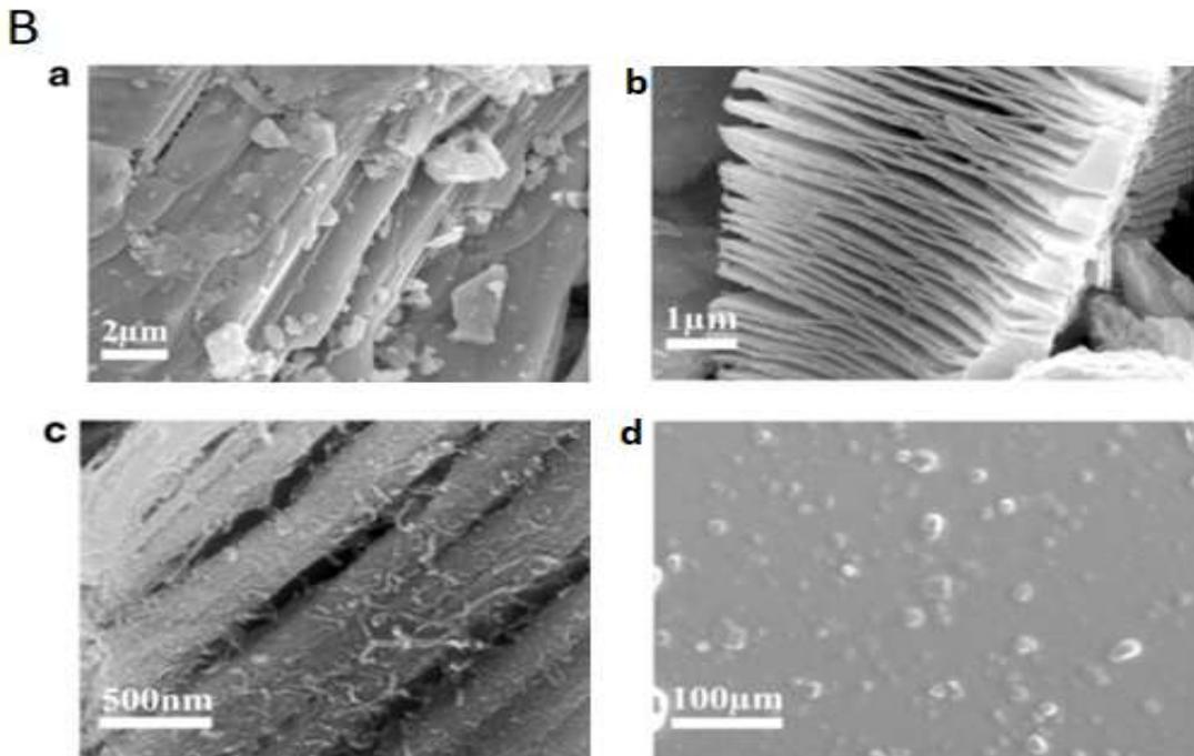
**Fig.4.** (A) Schematic demonstration of Ti<sub>3</sub>C<sub>2</sub> MXene and Ti<sub>3</sub>C<sub>2</sub>/MWCNT/Chit nanocomposite synthesis process. (b) SEM images of Ti<sub>3</sub>AlC<sub>2</sub> (a) before and (b) after treatment with HF; SEM images of (c) Ti<sub>3</sub>C<sub>2</sub>/MWCNT low magnification (d) Ti<sub>3</sub>C<sub>2</sub>/MWCNT/Chit composite. Reprinted by permission from Ref. [54]. Copyright 2020, Springer Nature.
