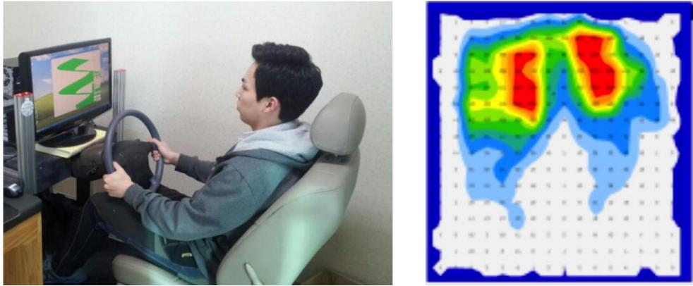
Fig 1. Experimental equipment A. driving simulator for steering accuracy, B. Result of Force Sensitive Matrix array for seating symmetry
