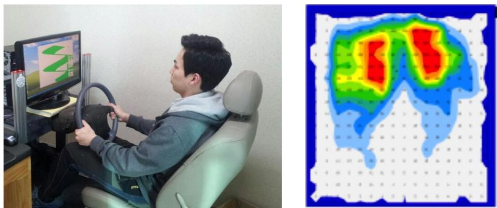
Fig 1. Experimental equipment A. driving simulator for steering accuracy, B. Result of Force Sensitive Matrix array for seating symmetry
