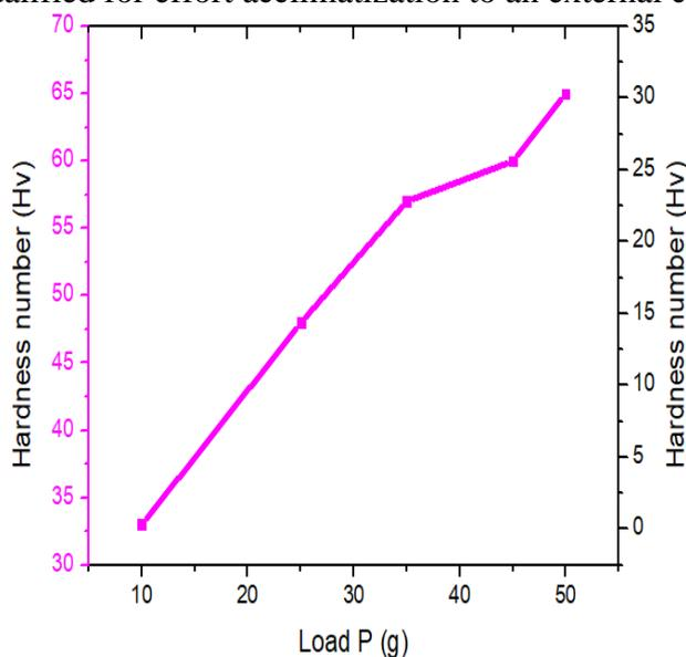
**Fig.8. exposed load of Vickers hardness crystal of L-LMhCl – CA.**
