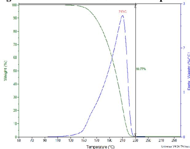
Fig. 6 L-LMHCl – CA of TG/DTA curve.
