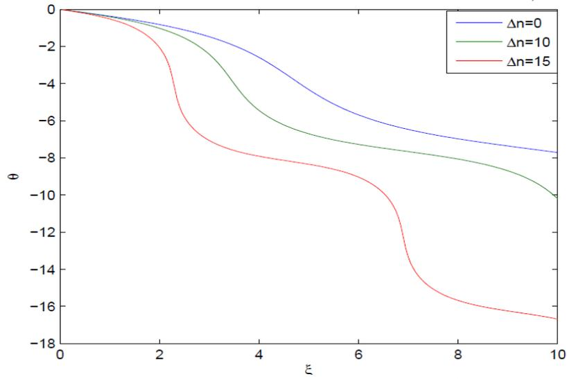
Figure 11. Effect of channel depth on axial phase shift of laser beam.
