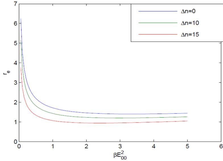
Figure 8. Effect of channel depth on self trapping of laser beam.
