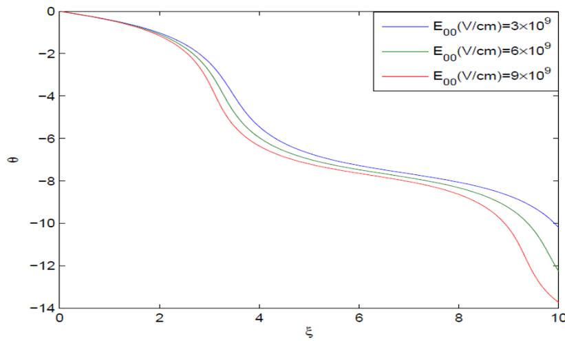
Figure 12. Effect of laser field amplitude on its axial phase shift.
