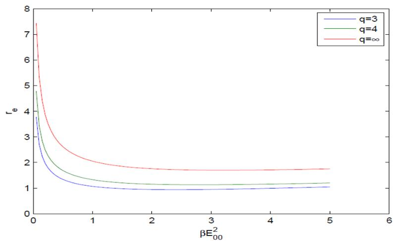
Figure 7. Effect of deviation parameter q on self trapping of the laser beam.
