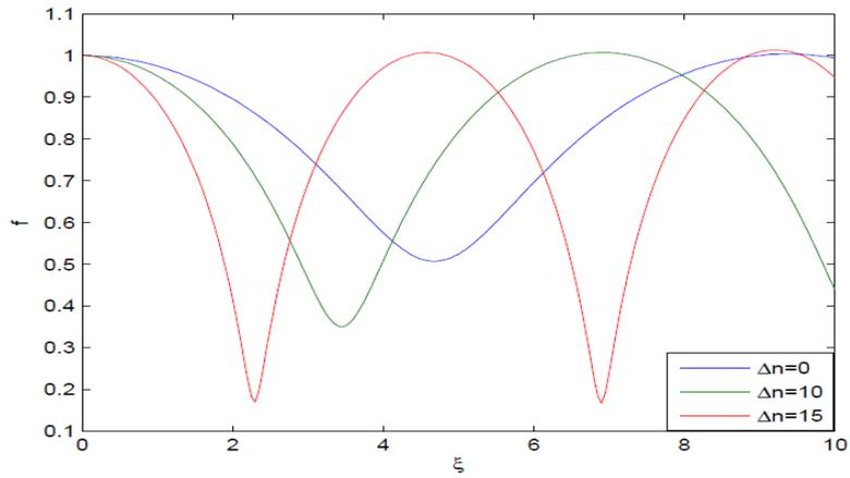
Figure 5. Effect of channel depth on self-focusing of laser beam.
