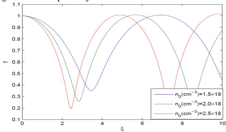
Figure 4. Effect of plasma density on self-focusing of laser beam.
