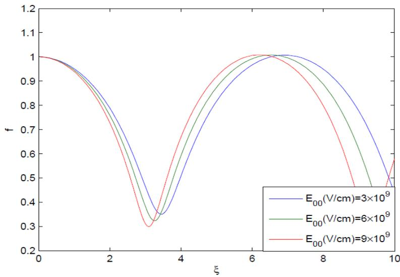
Figure 6. Effect of laser field amplitude on its self-focusing
