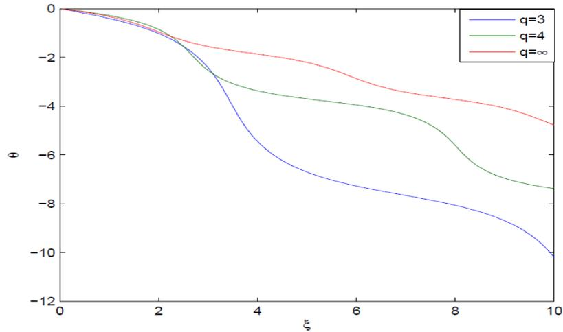
Figure 9. Effect of deviation parameter q on axial phase shift of laser beam.
