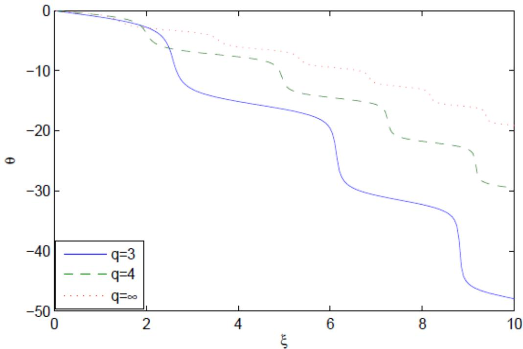
Fig.1. Effect of q on axial phase of laser beam.
