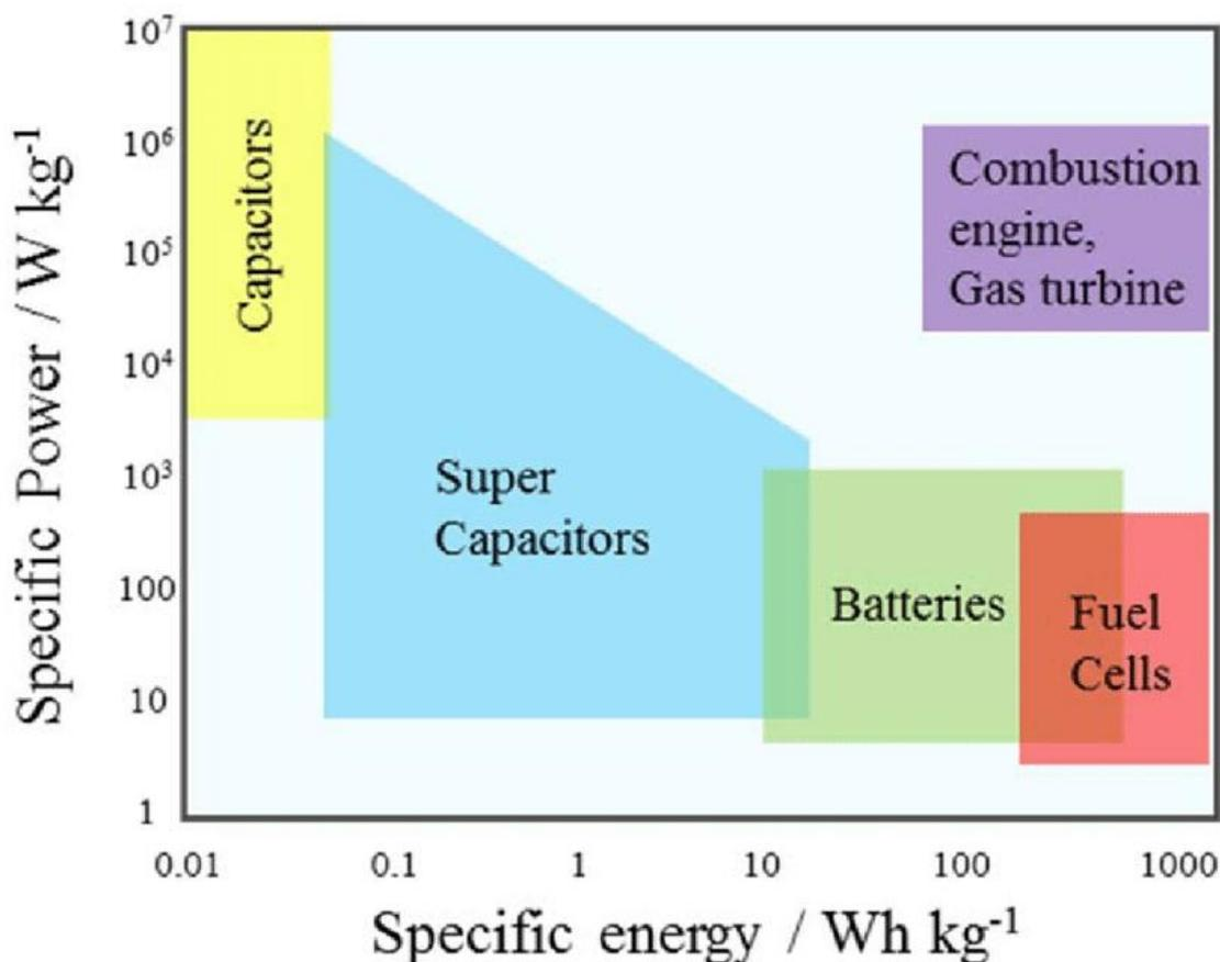
Fig. 2: Simplified Ragone plot for the various electrochemical energy conversion systems.
