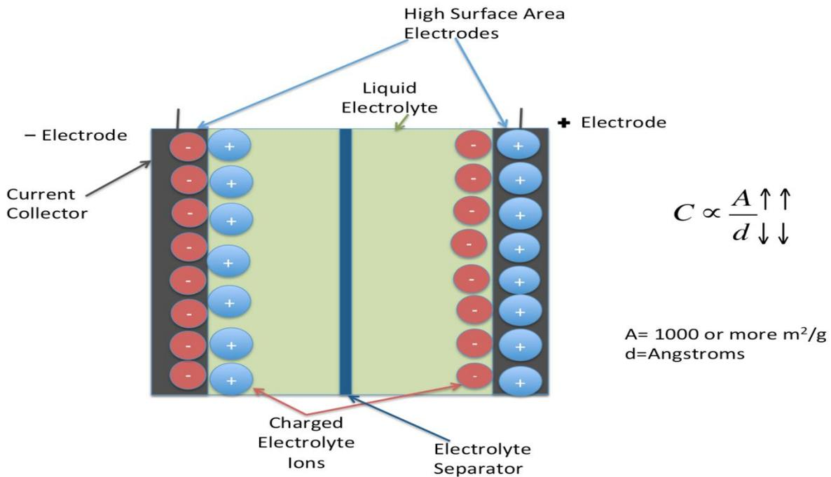
**Fig. 1: Schematic Diagram of Supercapacitors**
