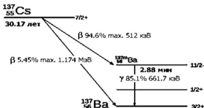
**Figure 3 Simplified scheme for the decay of cesium-137.**
