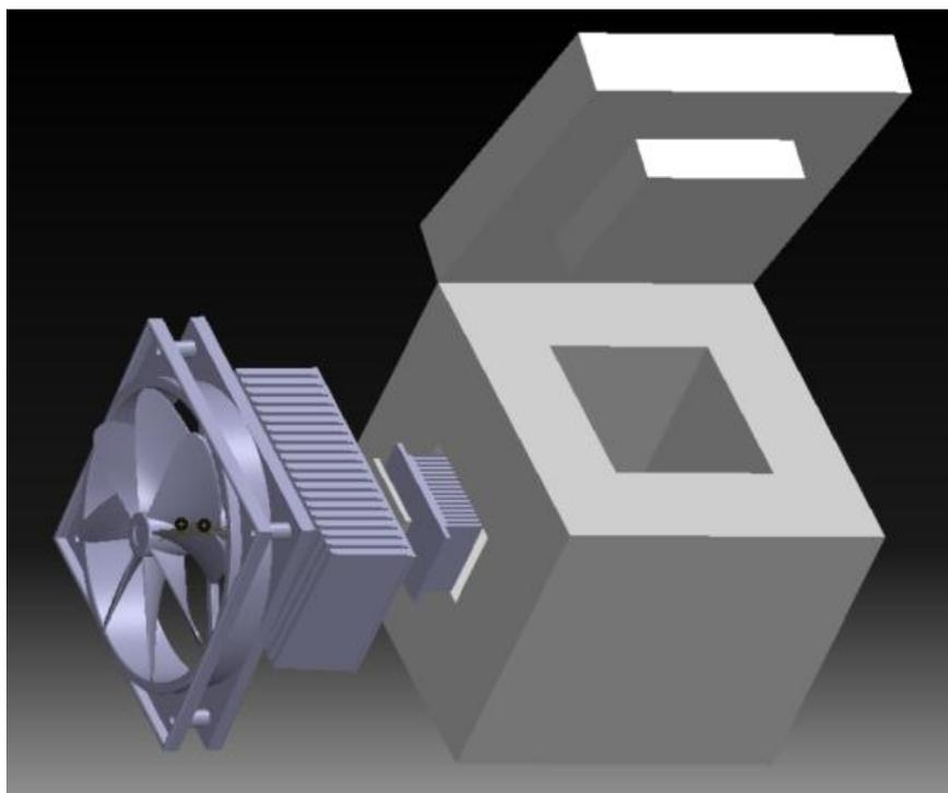
**Fig 3 Exploded view of cold box**
