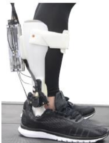
Figure 1: Existing exoskeleton model for Ankle-Foot Orthosis (Yufeng Zhang et al. [1])
