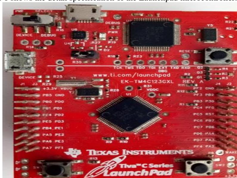
Figure 4: TIVA C series Launchpad Arduino microcontroller
