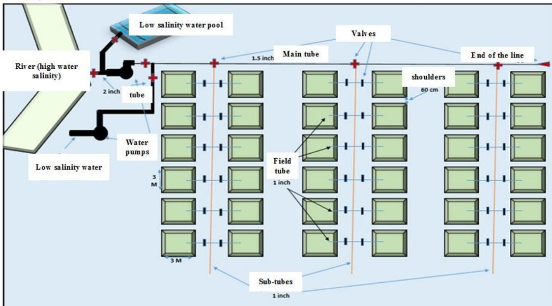
Figure (1) Scheme of the field experiment and the washing system used in the washing experiment.
