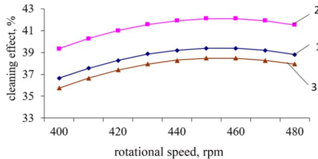
Figure.5. Graphs of changes in the cleaning effect depending on the frequency of rotation of the peg drum
