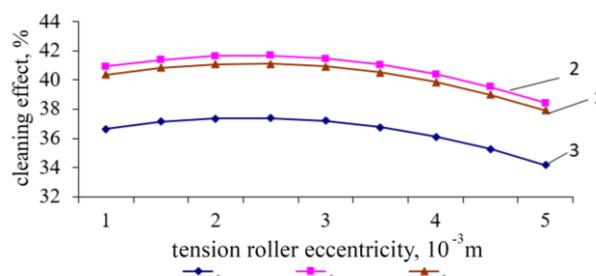
Figure.6. Graphs of the change in the cleaning effect depending on the eccentricity of the tensioning roller with an elastic element
